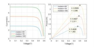
Figure 6: I-V and P-V characteristics of Single cell PV model using Sim Electronics Simulation Model
