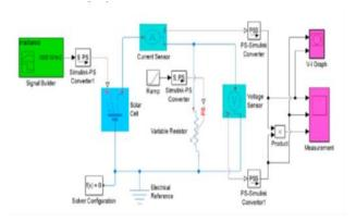
Figure 5: Simulation Model for a single Cell
