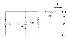
Figure 2 Practical one diode model for solar cell.
