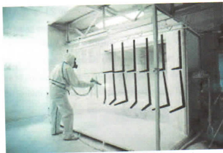
Fig.1.1 Conventional powder coating method
