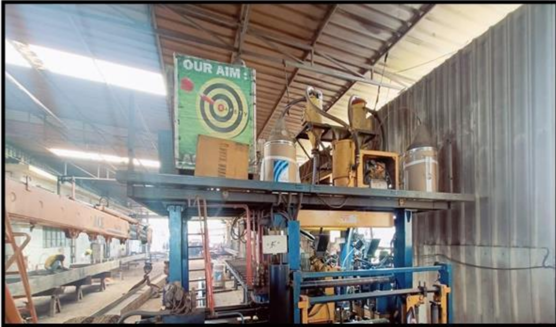
Figure 5: Students are taking information about Submerged-arc welding (SAW) and learning the use of Submerged-arc welding (SAW).
