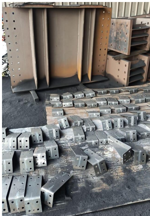
Figure 6: Components used to joined steel members
