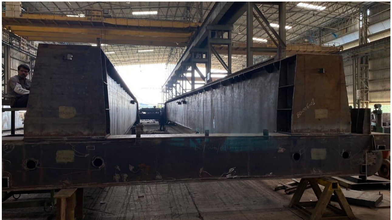
Figure 9: Components of Gantry Girder
